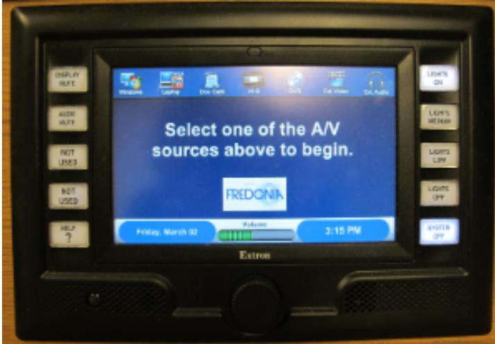
1. The Extron Touchpanel has buttons on the sides for light control, muting, and system off. There is also a volume knob located at the bottom.
