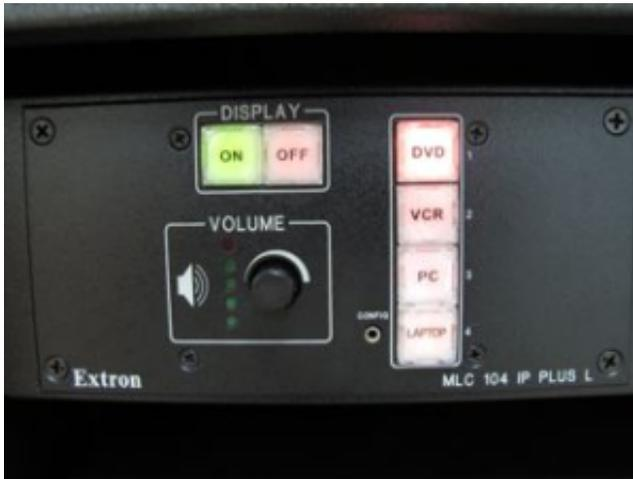
1. Push the "ON" button to start the projector.\* Pull the screen down.
